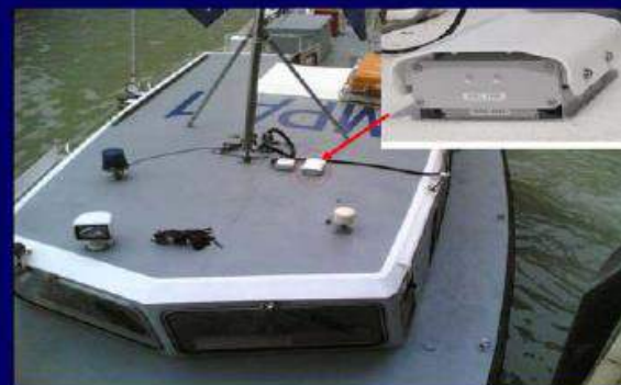
A TYPICAL INSTALLATION OF PORTABLE HARTS TRANSPONDER ONBOARD HARBOUR CRAFT
